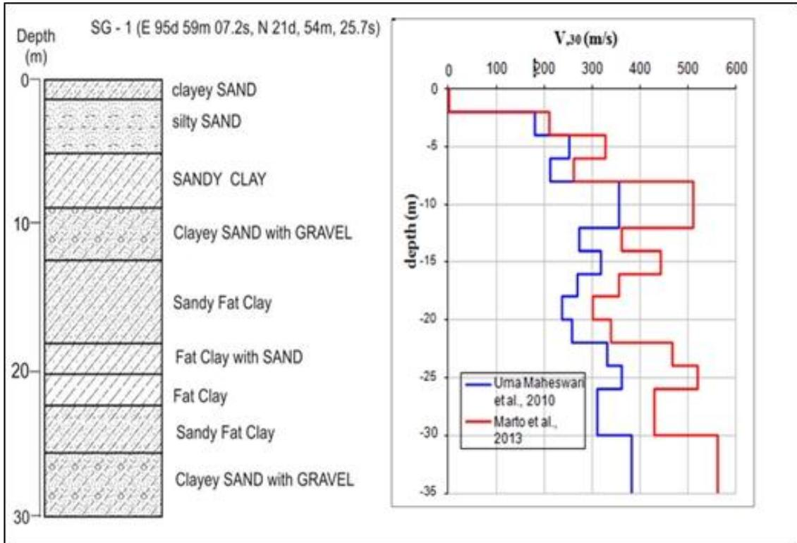
Figure (1.5) Soil profile and shear wave velocity profile ( $V_s 30$ ) by using corrected  $N$  value for SG-1
