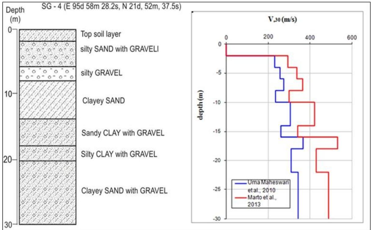
Figure (1.8) Soil profile and shear wave velocity profile ( $V_s 30$ ) by using corrected N value for SG-4
