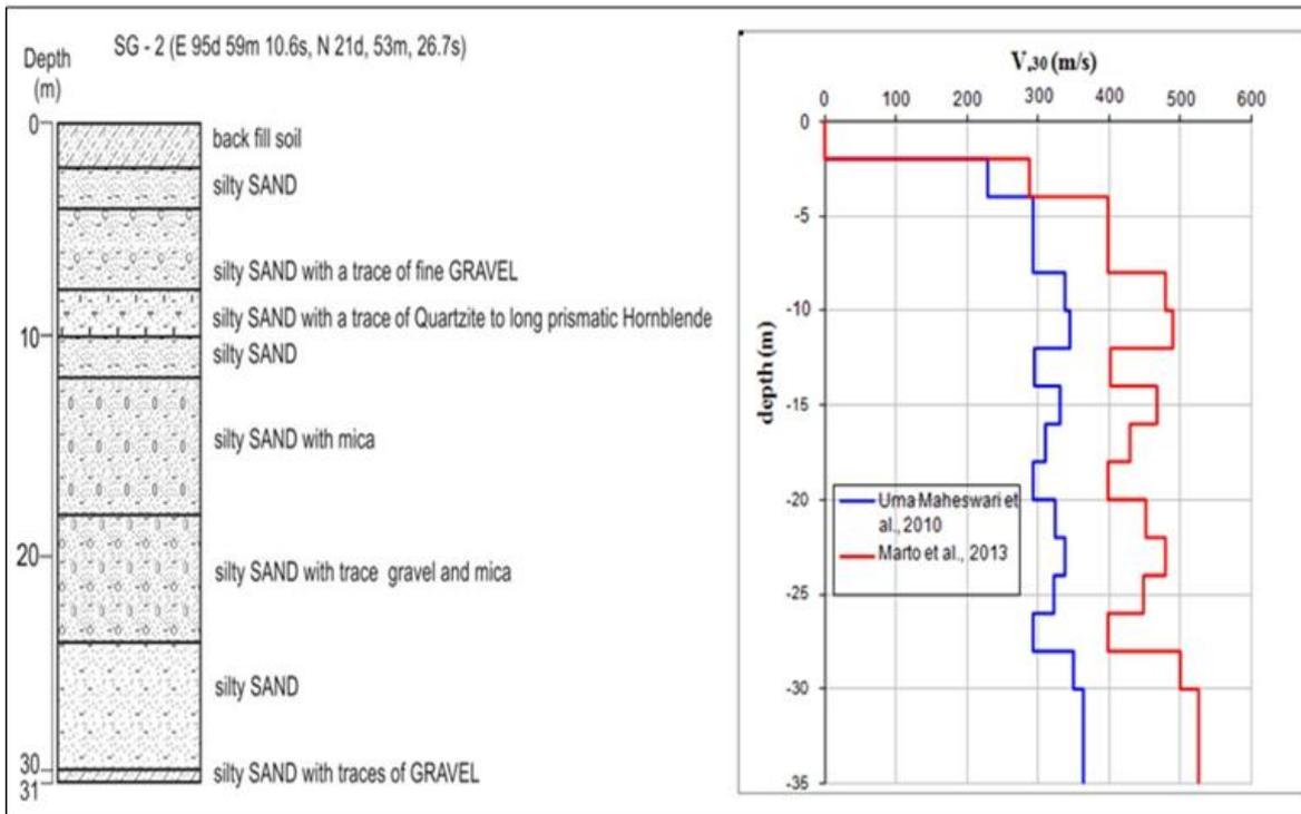
Figure (1.6) Soil profile and shear wave velocity profile ( $V_s 30$ ) by using corrected N value for SG-2
